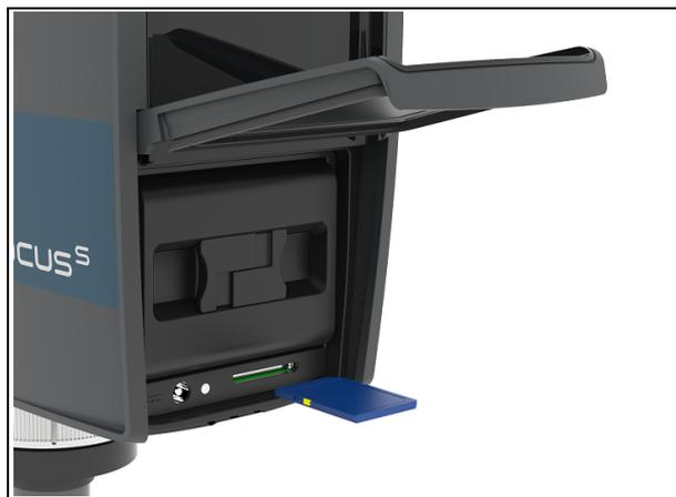
Figure 6-8: Inserting the SD Card
