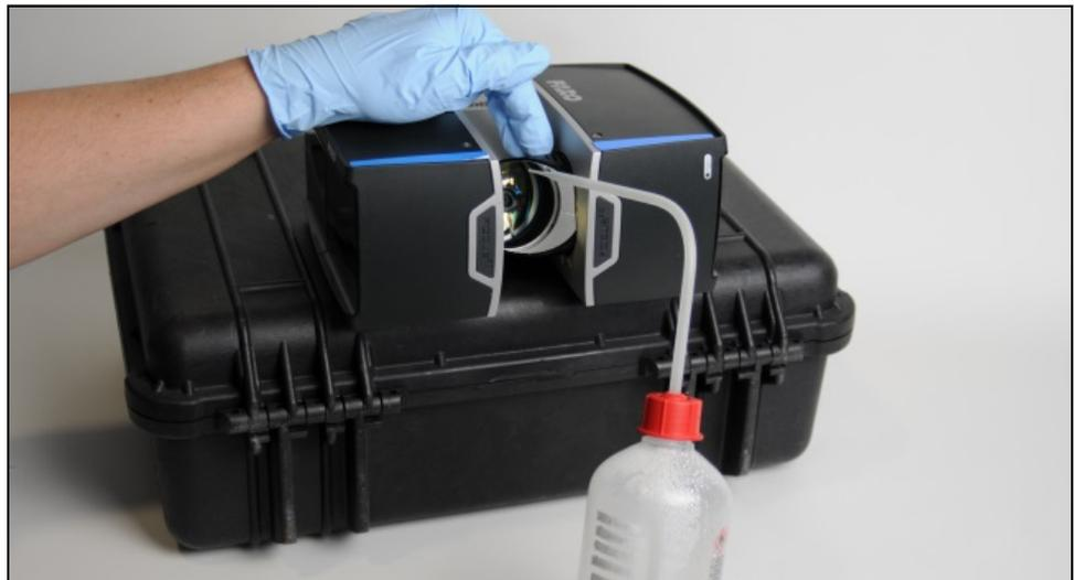
*Figure 9-14: Cleaning mirror module or sensor cover*
