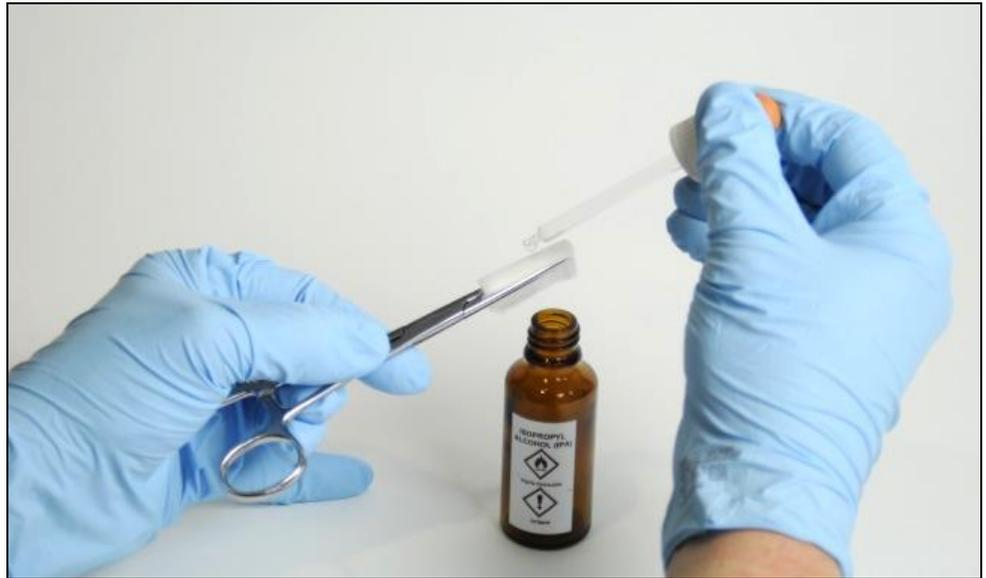
*Figure 9-8: Soaking the cleaning pad*
