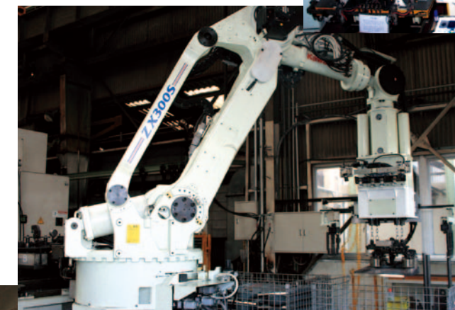
Releasing and loading / unloading of large-sized workpieces by vision system
